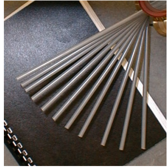
Fig. 6. Evolving eye morphology. (a) Top view of the setup of the experiments. The robot is equipped with a number of tubes that can be moved under program control. Light sensitive diodes have been placed at the inner end of the tubes (which mimic the facets) to ensure that a particular aperture is maintained. The vertical light tube represents the obstacle. (b) One distribution of the facets. The non-uniform spacing is clearly visible.
